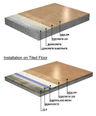
**SYSTEM CONFIGURATION** • The *TopCrete 220* micro topping system is very versatile and may be applied in any number of coats and techniques to achieve a variety of effects. A recommended system
